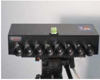
3DTV's camera rig has eight lenses and sensors.
